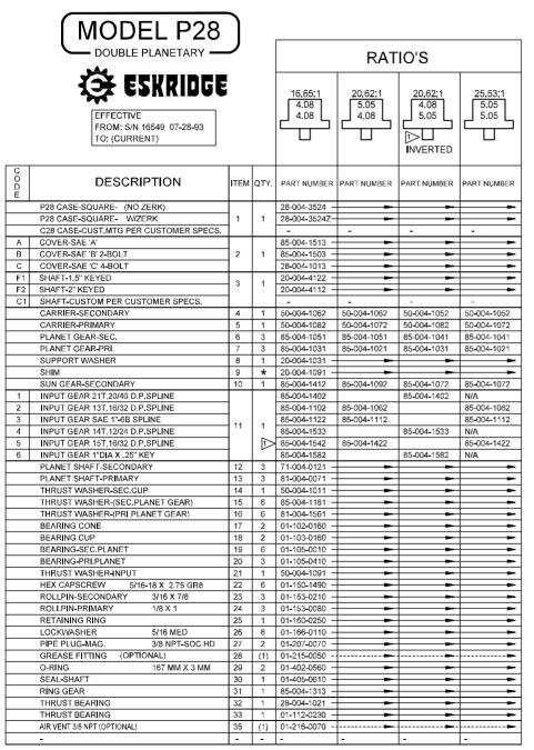
NOTE **\*** BEARING PRELOAD DETERMINES QUANTITY OF SHIMS.
