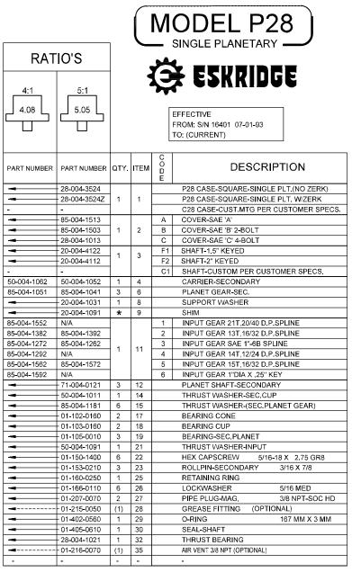
NOTE \* BEARING PRELOAD DETERMINES QUANTITY OF SHIMS. SEAL KIT; P/N 20-016-0511; INCLUDES ITEMS 29 AND 30.
